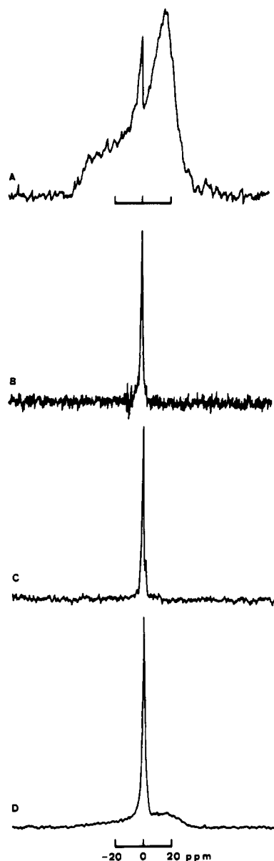
FIGURE 3: Proton-decoupled ^{31}\text{P} powder NMR spectra of unsonicated, aqueous dispersions of the \text{NH}_4^+ salt of 1,2-dipalmitoyl- sn -glycero-3-phospho-L-serine recorded at 42^\circ\text{C} on a Bruker CXP 300 NMR spectrometer operating at 121.47 MHz. (A) ^{31}\text{P} powder pattern of an unsonicated dispersion (100 mg/mL = 0.133 M) in \text{H}_2\text{O}/^2\text{H}_2\text{O} (1:1 v/v), apparent pH 6.9. (B) The above dispersion was made alkaline, pH \approx 12 , by adding NaOH. (C) Crystals of the protonated form of the same phospholipid were dispersed at 100 mg/mL (0.133 M) in \text{H}_2\text{O}/^2\text{H}_2\text{O} (1:1 v/v) at 70^\circ\text{C} to an apparent pH of 3.7. The pH of this suspension was adjusted to 11.2 by adding NaOH, and the spectrum was recorded. (D) The same dispersion as described under (C) after returning the pH to 6.8.
